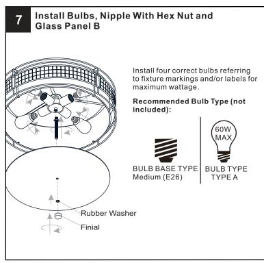
**IMPORTANT**: This CONVERTIBLE fixture can be mounted as pendant light or semi-flush light. **DO NOT CUT SUPPLY WIRES** if you intend to use it as pendant light.
