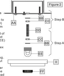
the Nipple (DD) into the Crossbar (AA) until the Nipple (DD) is about 0.375" above the Crossbar (AA).
